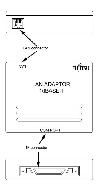
Figure 1.1 10BASE-T LAN adapter
